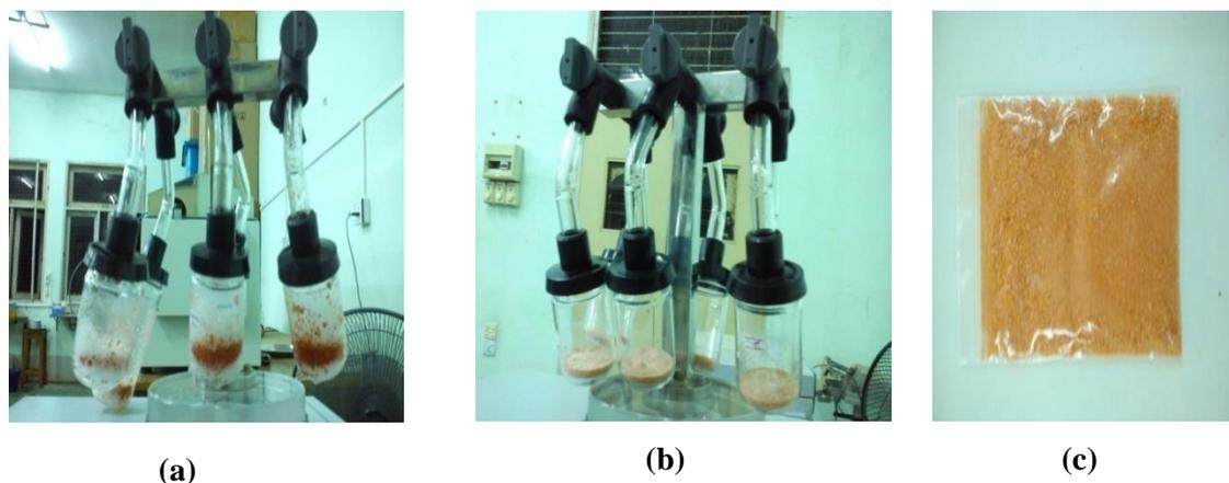
**Figure (1) (a) (b) Freeze-dried Processing of Tomato Juice Powder and (c) Prepared Tomato Juice Powder Sample**
