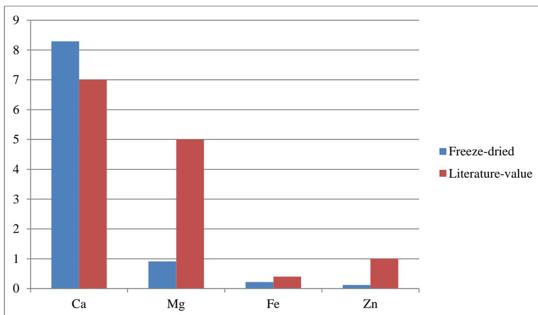
**Figure (5) Elements Content (w/w %) of Freeze-dried Tomato Juice Powder by X-ray Fluorescence Spectrometry (XRF)**
