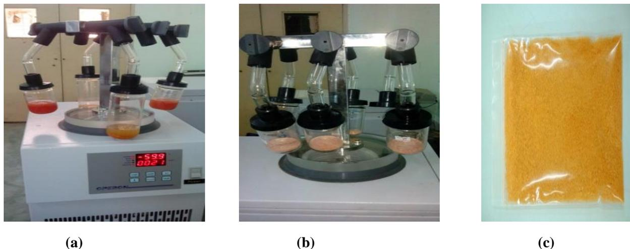
**Figure (2) (a) (b) Freeze-dried Processing of Carrot Juice Powder and (c) Prepared Carrot Juice Powder Sample**
